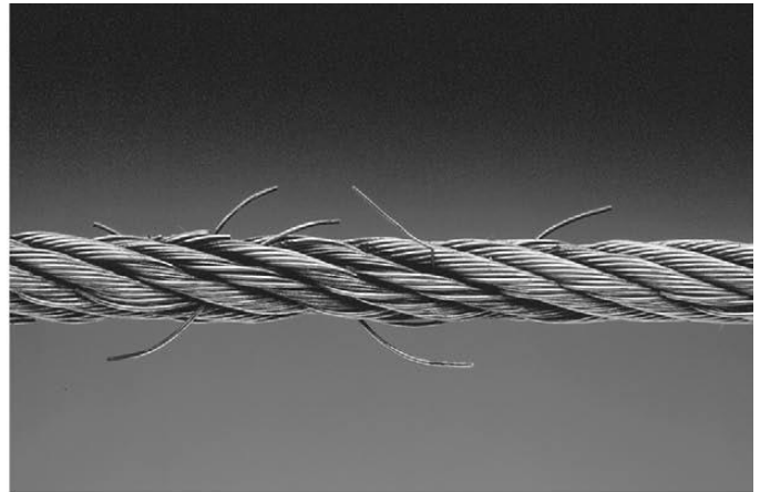
Cable With Broken Wires
