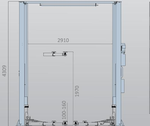
Minimum Concrete Requirement 150mm Recommended Ceiling Height 4.6m Power Requirements 3.5kw 9 amps Fast motor No neutral required Freight Dimensions 433 x 57 x 93cm 895kg
