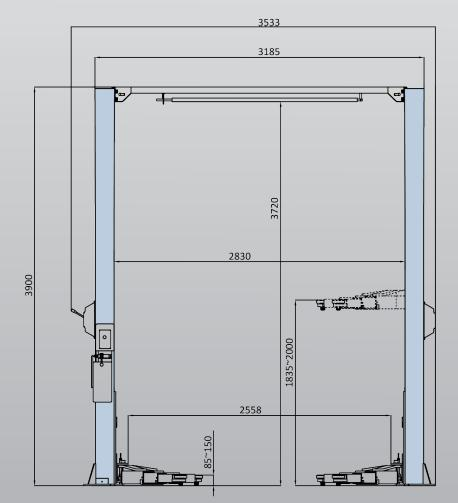
**Minimum Concrete** Requirement 115mm Recommended **Ceiling Height** 4.2m **Power Requirements** 240v 2.2kw 16 amps 3 phase 3.5kw 9 amps Fast motor Neutral required **Freight Dimensions** 391 x 57 x 110cm 686kg
